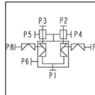
Sterile Filter Shunt Valve with Condensate Drain Valves
