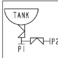
Tank Bottom Valve with CIP/SIP Valve
