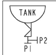
Tank Bottom Valve with CIP/SIP Port
