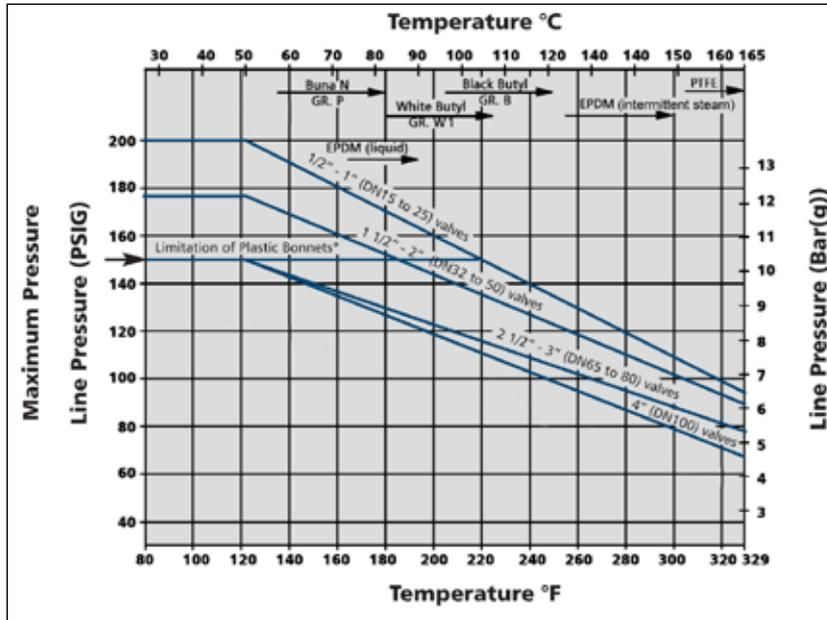
\* This line shows the limitation of plastic bonnets including the 963 and Advantage Actuators.
