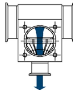
Example: 1.5" (DN40) Zero Static Tee with 3" (DN80) Run
