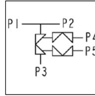
Zero Static with Upstream Sample and Downstream Purge
