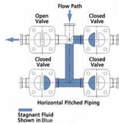
In case where process piping falls outside of FDA expectations, as noted from the High Purity Water Guide reference above, the owner of the system is expected to have special sanitizing procedures. These special sanitizing procedures can be costly in production time and processing cost and should be avoided whenever possible.
