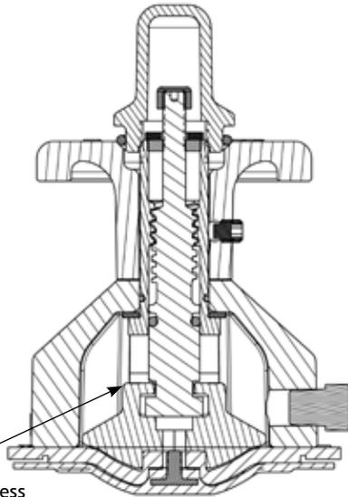
T-slot style compressor (stainless steel compressor version only)
