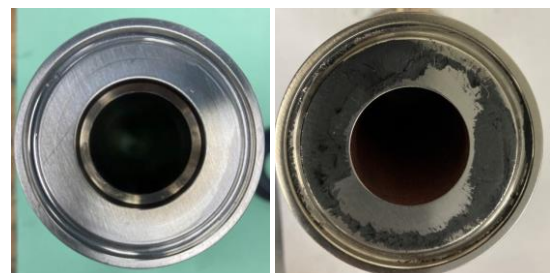
After exposure to 500 SIP cycles: Comparison of stainless steel flanges after removal of EPDM gaskets
