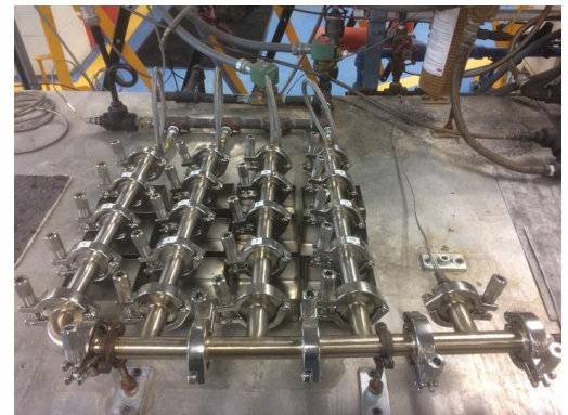
Steam-In-Place test stand for hygienic gaskets
