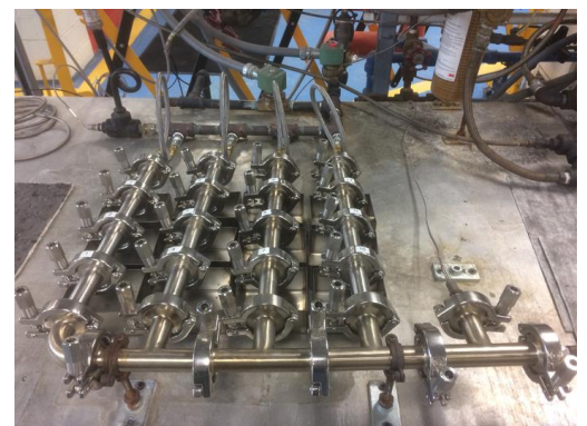
Steam-in-Place test stand for hygienic gaskets
