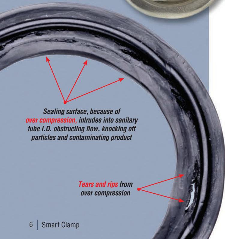
*Sealing surface, because of over compression, intrudes into sanitary tube I.D. obstructing flow, knocking off particles and contaminating product*
