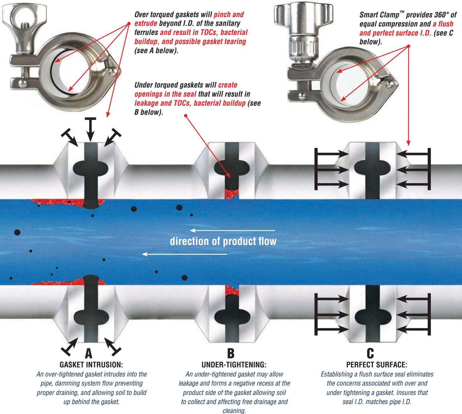
When a gasket is under-tightened, the result is a negative recess between the ferrules allowing soil and bacteria to accumulate and become entrapped (see B in illustration).
