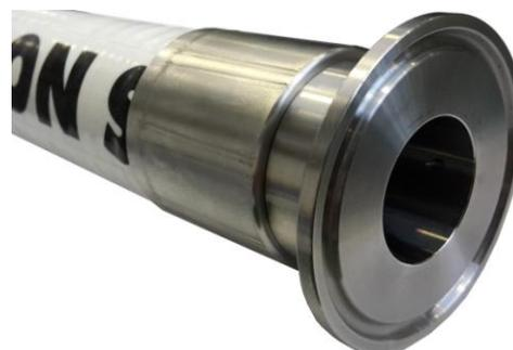
Aerrex offers a complete line of stainless steel fittings including hose assemblies. All Aerrex fittings are constructed from 316L stainless steel, have a standard surface finish of Ra<0,5 micron, and are secured to the hose by a collar with a 360° circumferential crimp.
